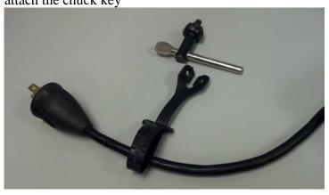
**Step 5:** Insert the long end of the chuck key into right ear of the chuck key holder.
