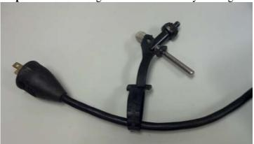
**Step 6:** Finally, insert the short side of the chuck key into the left ear. This will be difficult to do as well, but as you can see, it is possible.
