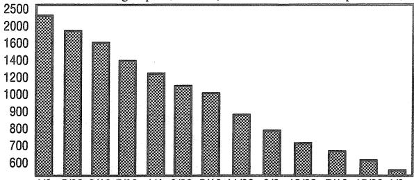
1/8 5/32 3/16 7/32 1/4 9/32 5/16 11/32 3/8 13/32 7/16 15/32 1/2 **Example:** 1/2" diameter drill bit should be run at 600 RPM. Speeds may be increased when drilling wood, composites, plastics, etc.
