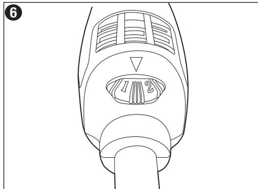
The numbered positions, 1 through 6 inscribed on the variable speed dial, do not indicate any precise speed but are good reference points. The higher the number, the higher the tool speed.
